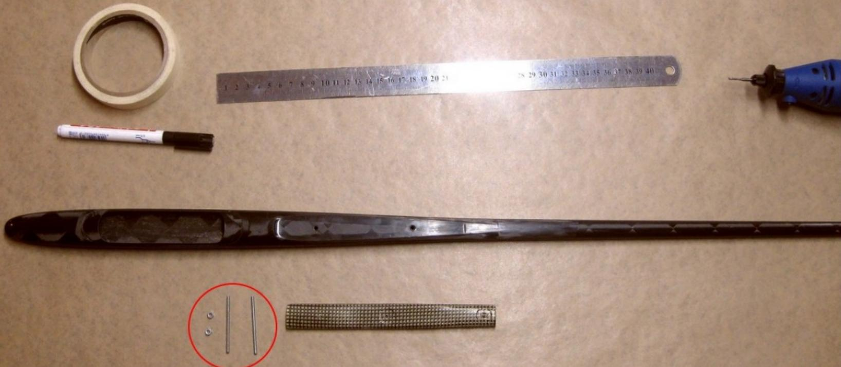
To install ballast chamber needs two stud-bolt or screw with nuts M3.
